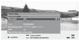
In the "Recorder" menu line, select "DR" for Digital Recorder with the arrow buttons ◆ ▶ . For "VPS", select whether or not VPS is to be used (if it is available). Enter the date and the recording time for the timer recording with the numeric buttons on the remote control. Select under recording type whether you want to make a recording once only, daily, Mon-Fri or weeklv.
